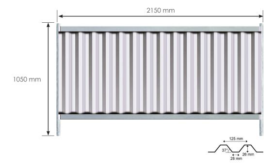
Block 'N' Mesh recommends using the 1 meter Blockade Construction Fence only in conjunction with Concrete Blocks or BraceBlok™ 50kg
